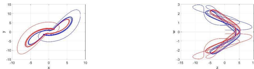
Figure 12. Phase plot of the new system (1), where we fix b = 10 and the initial condition X_0 = (0.2, 0.2, 0.2, 0.2) for blue color plot and Y_0 = (-0.2, -0.2, 0.2, -0.2) for red color plot. When a = 4.9 , the system (1) has coexisting period-2 attractors.
