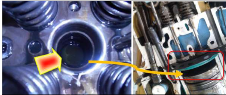
Figure 2. Solar is in the combustion chamber.
