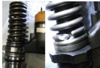
Figure 2. Spring injector broken.
